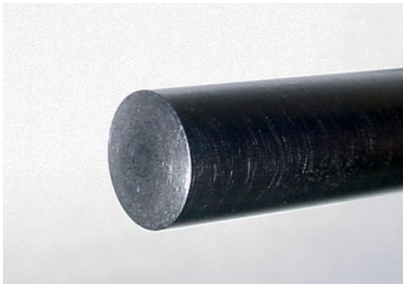
Photo – 4 Push Rod Exhibiting Normal Wear
