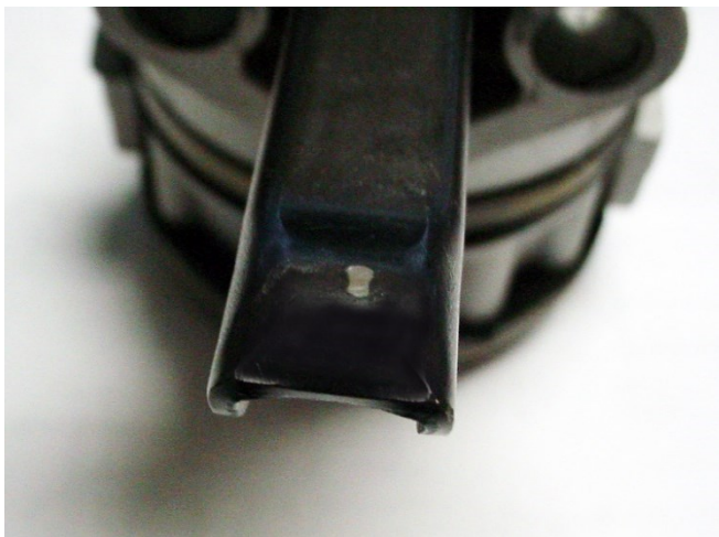
Photo – 2 Pump Lever Exhibiting Normal Wear
