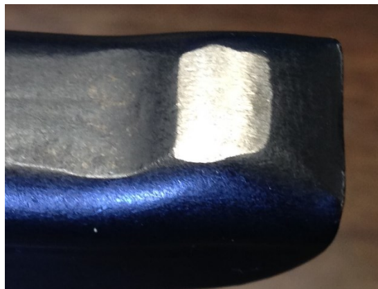
Photo – 6 Pump Lever from 62B Series Pump Exhibiting Abnormal Wear
