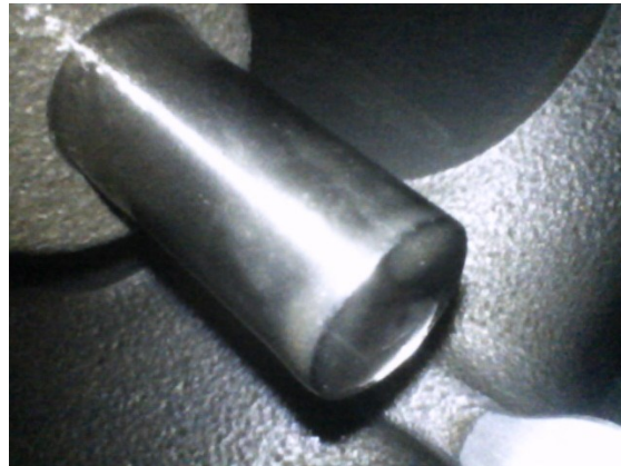
Photo – 3 Damaged Push Rod
