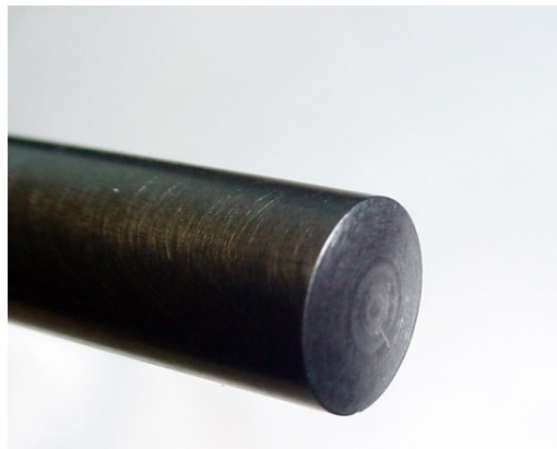
Photo – 4 Push Rod Exhibiting Normal Wear
