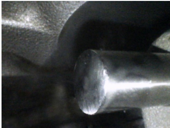
Photo – 3 Damaged Push Rod
